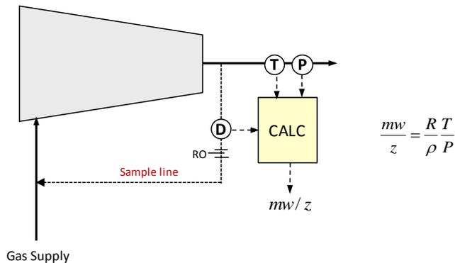
Unknown Composition - Using Compressor Performance to estimate mw/z
