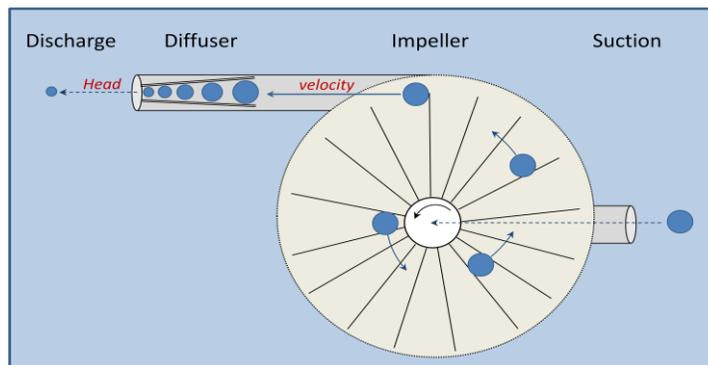
The kinetic energy of the gas leaving a radial impeller can be calculated from the impeller diameter and rotational speed. Ideal Head is the value of head that would result if all of the kinetic energy was converted to pressure potential energy.
